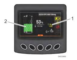
When the heater is active, the heater symbol (1) will appear.
