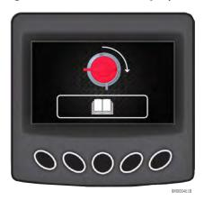
1. At machine start up a display reminding the user to engage the main contactor will be displayed.
