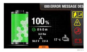
Once the battery balancing phase is complete, all hexagons will remain illuminated and the clock icon turns green.
